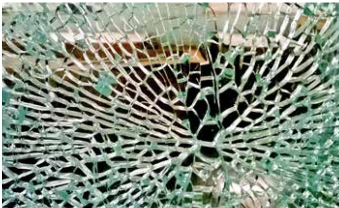
Image 2: The origin of breakage, caused by Nickel sulfide inclusions
